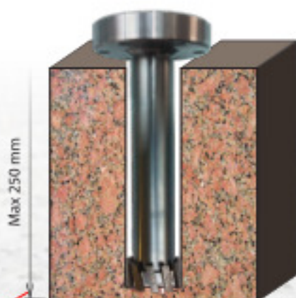
4. Ø40 STUBBING WHEEL Cut from 100 to 250 mm RPM: 4800 - 5500 Feed: 250 - 500 mm/min Each Step: 2 - 4 mm
