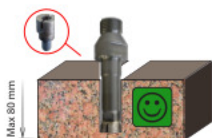
1. CROWN MILL Ø20 Cut from 30 to 80 mm RPM: 4200 - 4800 Feed: 800 - 200 mm/min Each Step: 2 - 3 mm
