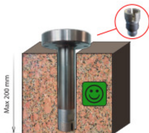
3. CROWN MILL Ø30 Cut from 60 to 200 mm RPM: 4200 - 4800 Feed: 250 - 500 mm/min Each Step: 1 - 3 mm
