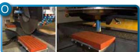
**Redressing Devices for Disc and Core Drill, including Automatic Management Software**
