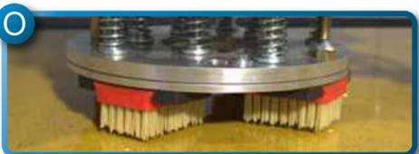
**Spring-Loaded Head for Surfaces Honing and Leathering**
