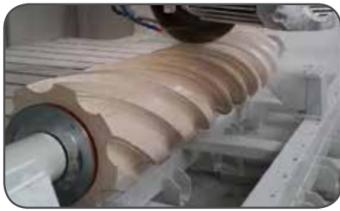
5-Axis Carving with Disc and Mill Bits
