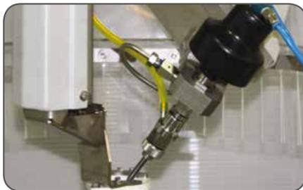
**5 Axis Piercing Cutting Head allowing Tilted cuts and Undercuts**
