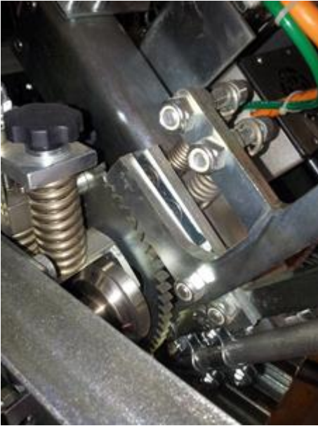
Head R-axis -90^{\circ} - +90^{\circ} in 5^{\circ} steps
