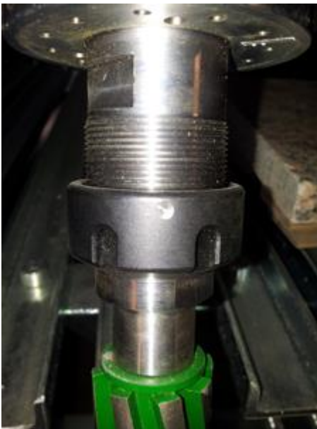
Spindle with ER32 collet and adapter 22,2 mm
