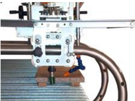
Pos. 1 0° profiling, drilling, drainboard
